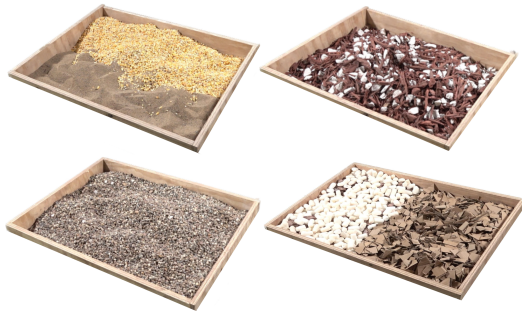
Fig. 4: Example terrains illustrating different compositions, materials, and topography. Top left: Partition of Sand and Corn. Top right: Mixture of Mulch and Gravel. Bottom left: Single of Pebbles. Bottom right: Layer of Shredded Cardboard (right), Packing Peanuts (left, top layer), and Slates (left, bottom layer).
