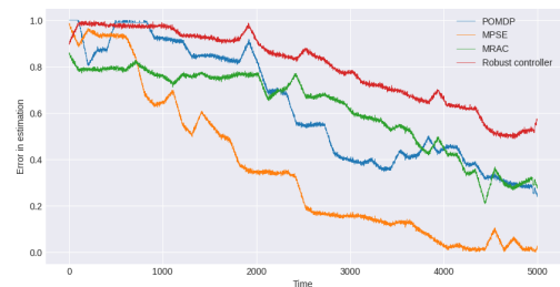
Fig. 2 Error evolution over time for the GUAM agent controlled by MPSE, POMDP with classical estimation, robust controller and MRAC.
