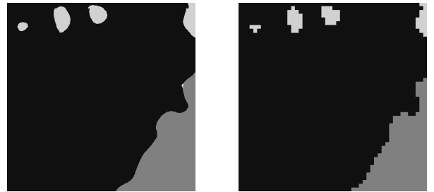
Fig. 1. The terrain map used as a state space in Section V-A. On the left is the original high-resolution Jezero crater map of terrain types. Each color represents a different terrain type: black terrain is benign, grey terrain is rough, and white terrain is rippled. The coarser 50 \times 50 grid used in simulations of Section V-A is given on the right.
