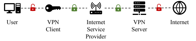
Fig. 1: Internet access via a virtual private network (VPN). VPN client encrypts the user data, and the internet service provider (ISP) cannot observe the user's traffic.
