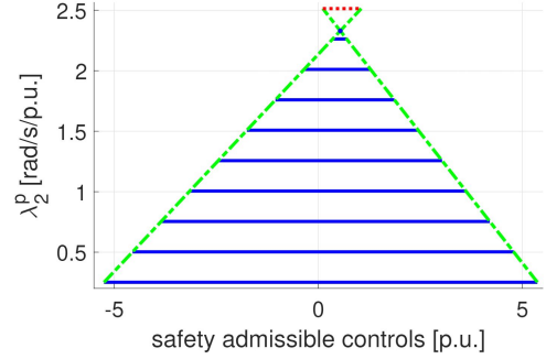
Fig. 2: Evolution of the interval of safety admissible controls in blue for the frequency of node 2. The blue dot corresponds to \lambda_2^{p*} . The green dash-dot lines correspond to \underline{u}_2^p(\lambda_2^p) and \bar{u}_2^p(\lambda_2^p) . The red dotted line indicates that \underline{u}_2^p > \bar{u}_2^p .
